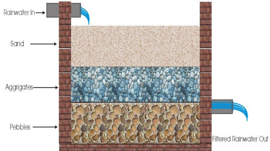
Figure No. 3.3 Design of Rainwater Harvesting Pit
