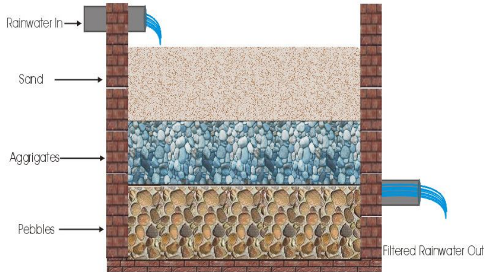
Figure No. 3.3 Design of Rainwater Harvesting Pit
