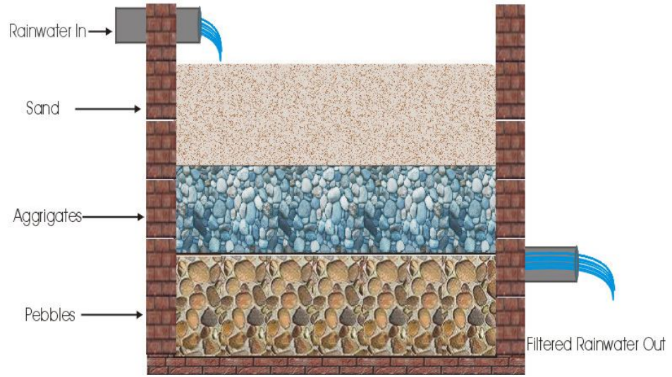
Figure No. 3.3 Design of Rainwater Harvesting Pit
